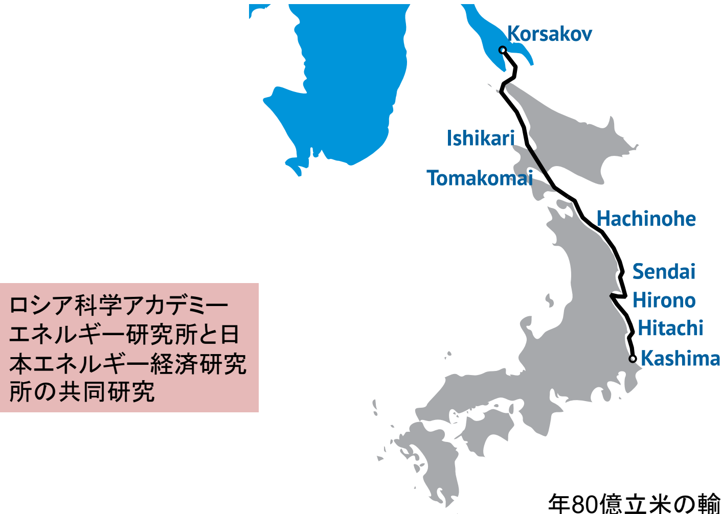
Figure 1. Proposed Subsea Pipeline Route*
