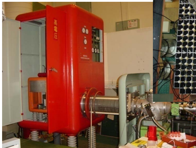
Pulsed neutron generator
